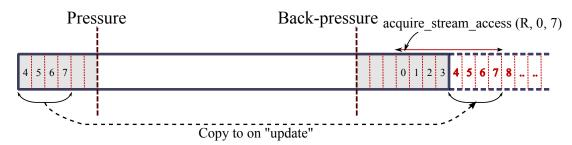
Figure 7.19: Allowing read accesses acquired as a range to overshoot the end of the stream buffer.
