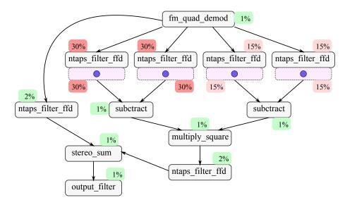
Figure 6.23: FMradio task graph and the proportion of computational load in each task.
