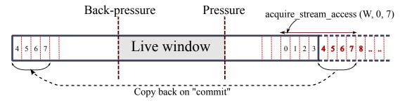
Figure 7.18: Allowing write accesses acquired as a range to overshoot the end of the stream buffer.
