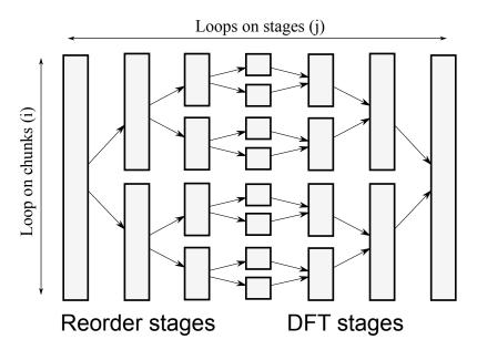
Figure 8.3: Data-flow graph for FFT.
